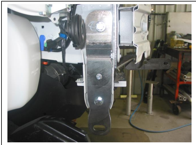
Figure 3: Install tow hook to passengers side
