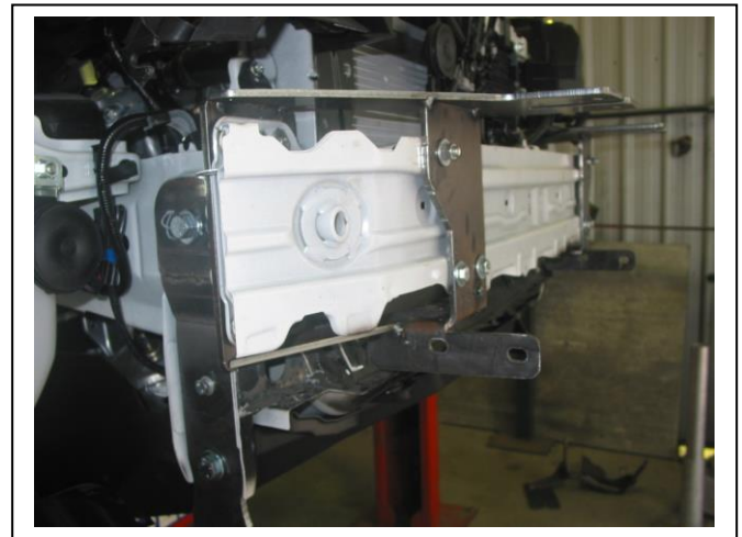
Figure 4: Install ECB mounts onto bumper support
