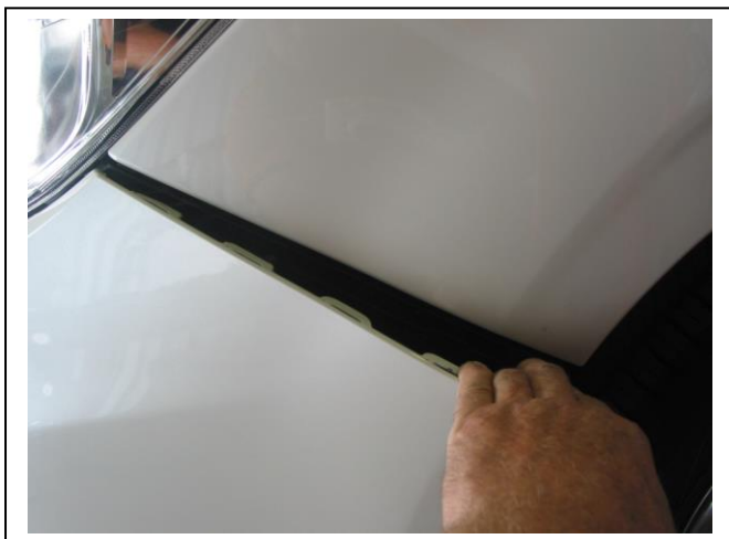
Figure 1: Unclip bumper from guard and light
